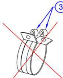
ATTENTION: the two edges of the band must remain in contact. The spacers (3) or anything else should NEVER be placed between them
